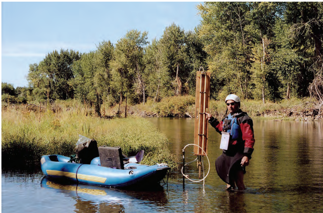
Figure 19. Hydrologist making a mini-piezometer measurement using a manometer board in the Parker reach of the Yakima River, Washington. (Photograph taken by William Simonds, U.S. Geological Survey, September 5, 2002.)
